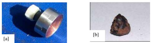
Figure 5– MFI EFP charge [a] and recovered fragment [b].
